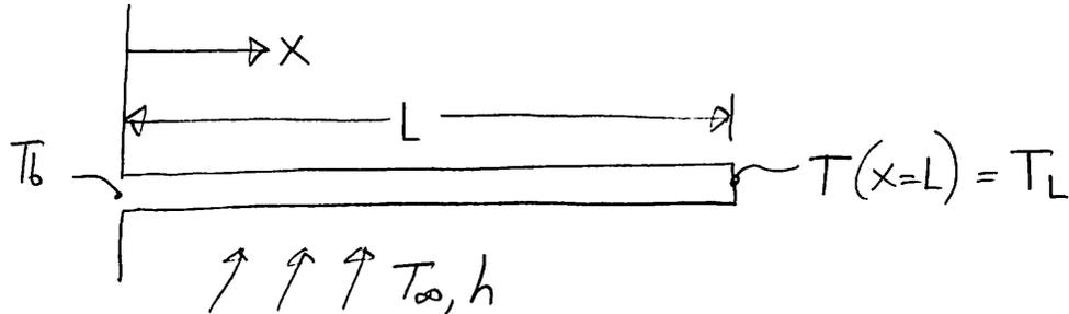
$$\frac{T - T_\infty}{T_b - T_\infty} = \frac{T_L - T_\infty}{T_b - T_\infty} \frac{\sinh(mx) + \sinh[m(L-x)]}{\sinh(mL)}$$
