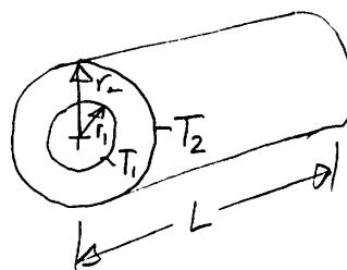
$$S_{cyl} = \frac{1}{k R_{cyl}} = \frac{2\pi L}{\ln(r_2/r_1)}$$
