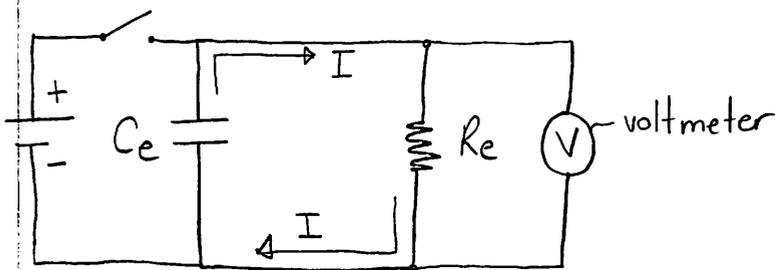
$$V(t) = V_0 e^{-\frac{t}{R_e C_e}} \quad \leftarrow \text{solution}$$
