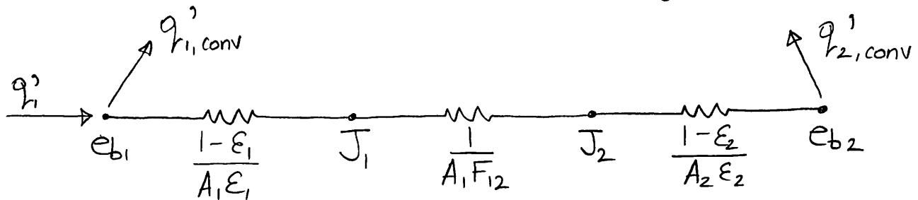
Since surface 2 is insulated :  $\text{q}_{h2,\text{rad}}' = \text{q}_{h2,\text{conv}}' \quad ①$
