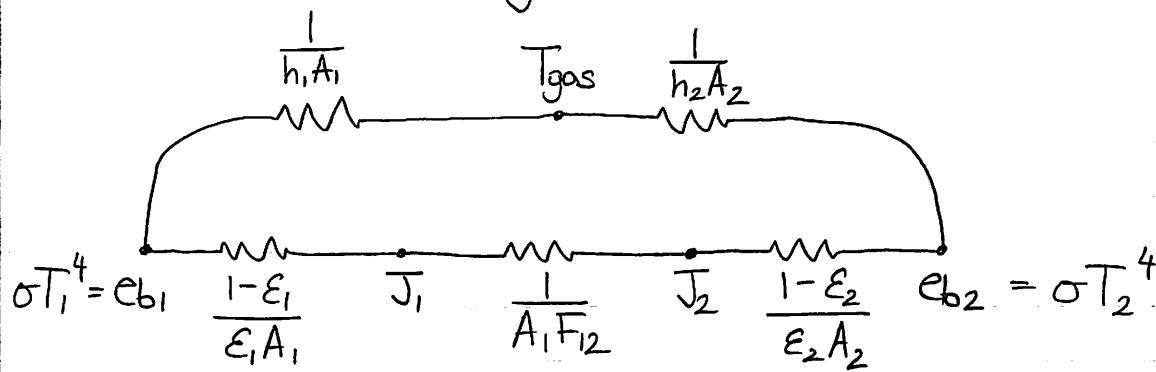
We need to solve this complete resistance diagram and it usually involves iteration since  $T_{\text{gas}}$  is unknown.
