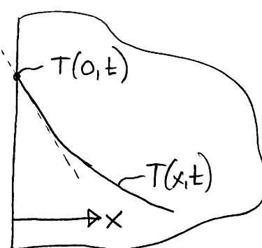
Example] Assume 1-D, steady-state, heat conduction through the axisymmetric shape below. Assume no heat generation & that it is well insulated on the outsides. Assume constant properties.
