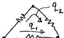
$$q_{L1} = (e_{b1} - e_{b2}) \left( \frac{1}{A_1 F_{12}} \right)^{-1} = -234.1 \text{ W/m}$$
