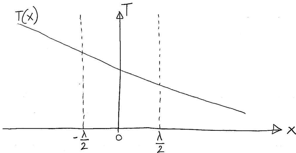
$$\dot{q}_{x+}'' = n m c_p \bar{c} T \left( x - \frac{\lambda}{2} \right) , \text{ where}$$
