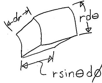
$$\begin{aligned} dS_1 &= dr \\ dS_2 &= r d\theta \\ dS_3 &= r \sin\theta d\phi \end{aligned}$$
