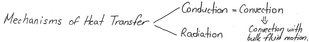
$$\dot{q}_x'' = -k \frac{\partial T}{\partial x} , \text{ where } k = \text{thermal conductivity [W/m·K]}$$
