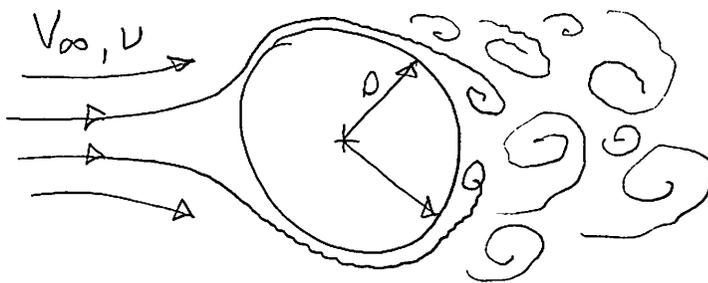
Turbulent boundary layer with separation.
