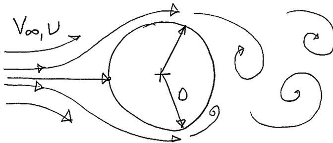
Note, Laminar flow with separation of the laminar boundary layer.
