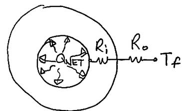
$$\pi a^2 L \dot{Q}''' = \frac{T_a - T_f}{\frac{\ln(b/a)}{2\pi L k_i} + \frac{1}{2\pi b L h}}$$
