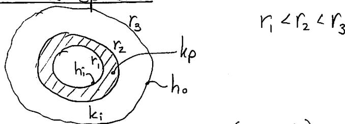
$$R_{\text{TOT}} = \frac{1}{4\pi r_1^2 h_i} + \frac{\left(\frac{1}{r_1} - \frac{1}{r_2}\right)}{4\pi k_p} + \frac{\left(\frac{1}{r_2} - \frac{1}{r_3}\right)}{4\pi k_i} + \frac{1}{4\pi r_3^2 h_o}$$
