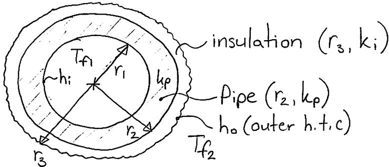
$k_i$  = insulation thermal c. $h_p$  = pipe thermal cond. $T_{f,i}$  = inner fluid temp. $T_{f,2}$  = outer fluid temp. $h_o$  = outer h.t.c. $r_1 < r_2 < r_3$
