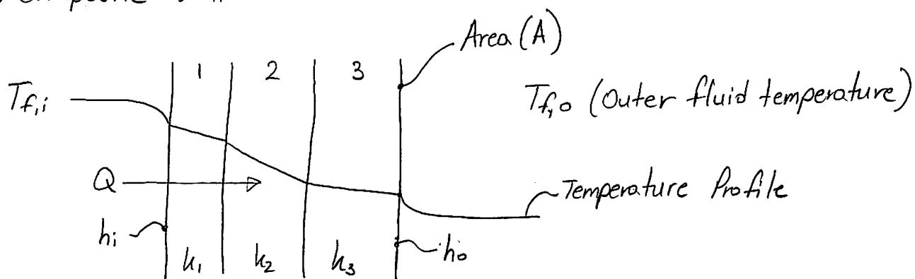
$$Q = \frac{A (T_{f,i} - T_{f,o})}{\frac{1}{h_i} + \frac{1}{h_o} + \sum_{j=1}^n \frac{L_j}{k_j}}$$
