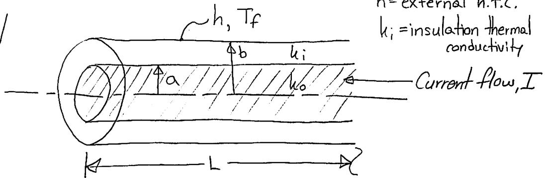
We have the wire electrical resistance,  $R_e$ , and the current,  $I$ , what is  $T_{max}$ ?
