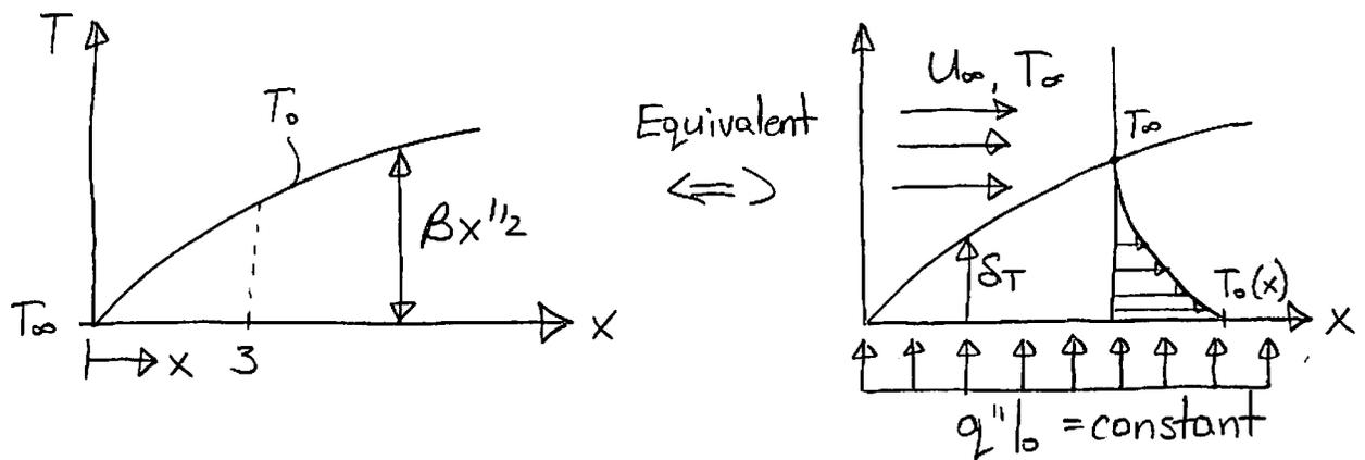
So now you know how the wall temperature varies for a prescribed uniform heat flux b.c.  $\Rightarrow$  its  $T_0 \sim \sqrt{x}$
