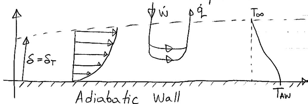
Note, the shear-to-thermal and kinetic-to-thermal energy conversion processes are fundamentally different. The shear mechanism is an irreversible process. Usually, most real cases involve both.
