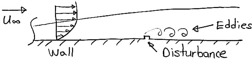
Note, these "disturbances" need not be physical. They may be fluctuations in the free stream velocity ( $U_\infty$ ), pressure gradient ( $\partial P / \partial x$ ), or very small scale surface roughness.
