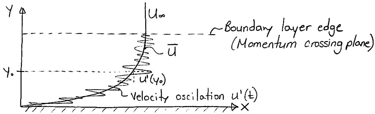
The average shear stress at any  $y$ -location in the turbulent region is:
