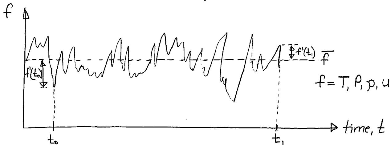
$$f = \bar{f} + f' \Rightarrow \bar{f} \equiv \text{mean component (time averaged)} \\ f' \equiv \text{fluctuating component (time dependent)}$$
