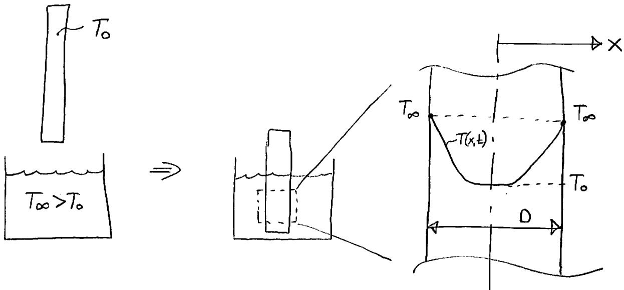
Assuming that the bar surface temperature assumes the fluid temperature instantaneously. What is the time required for the thermal front to penetrate the plate, i.e. the time for the center of the plate to "feel" the heating imposed on the outer surfaces.
