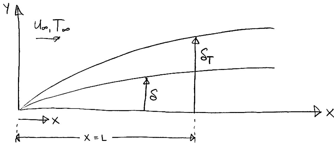
So when you say:  $Nu_L = \frac{hL}{k_f} = \frac{\text{convection h.t. at location L}}{\text{conduction h.t. of a water slab of thickness L}}$
